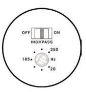
detected, rotate the input sensitivity control counterclockwise until it is eliminated and/or rotate the highpass crossover control clockwise to raise the crossover point.
